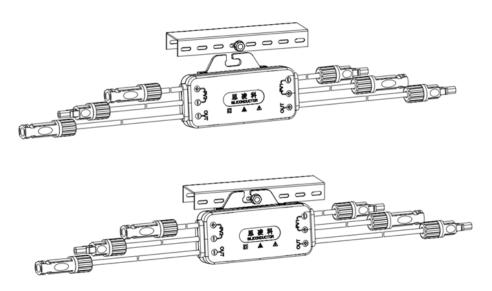
Option 2: Mounted on the PV module frame, snap the shutdown devie back plate onto the frame and make sure it is tightened in place.
